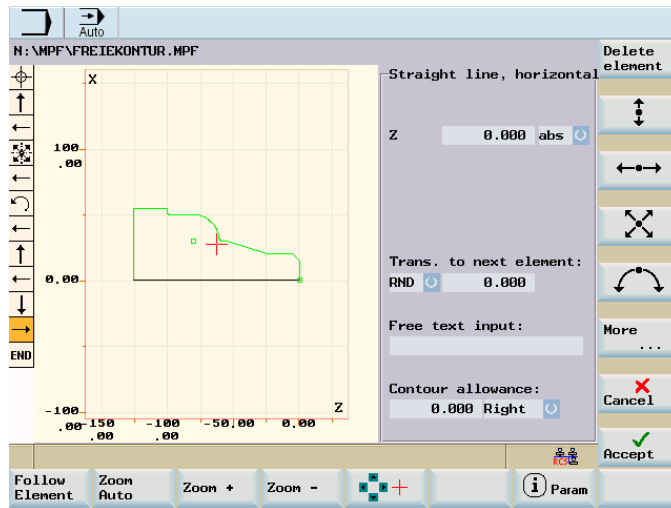
Figure 7-29 Edit a contour element
